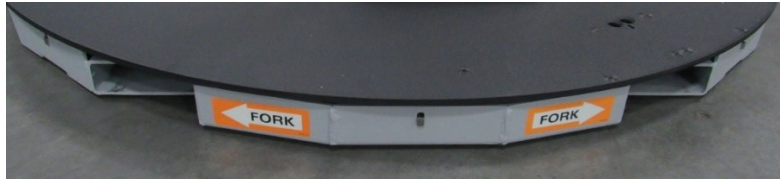
Illustration 2 - Machine Lifting Fork Pockets
