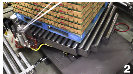
As wrap cycle begins, ropes held in place as turntable rotates.
