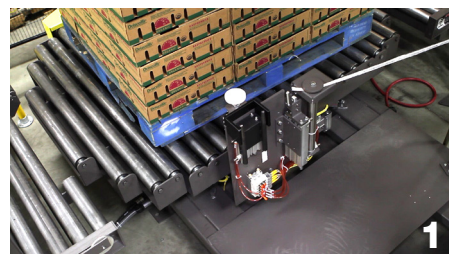
Two film ropes are held securely in the pneumatically operated clamp & cut mechanism.
