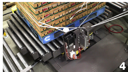
Clamp rods retract holding film ropes in place in preparation for film cutting.
