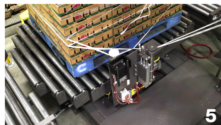
Cutter mechanism extends then retracts to sever the twin film ropes.
