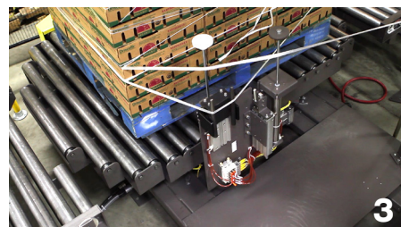
Near end of wrap cycle, 2 consecutive ropes are captured by clamp rods.
