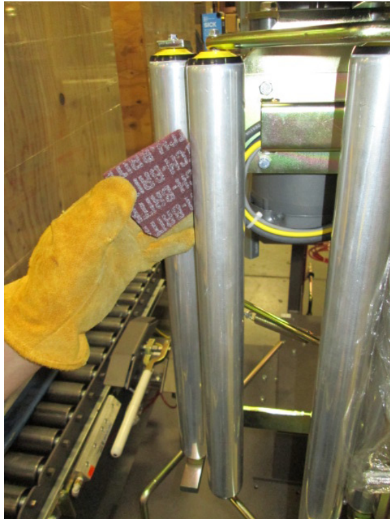
Figure 5 - 2 Cleaning Aluminum Rollers
