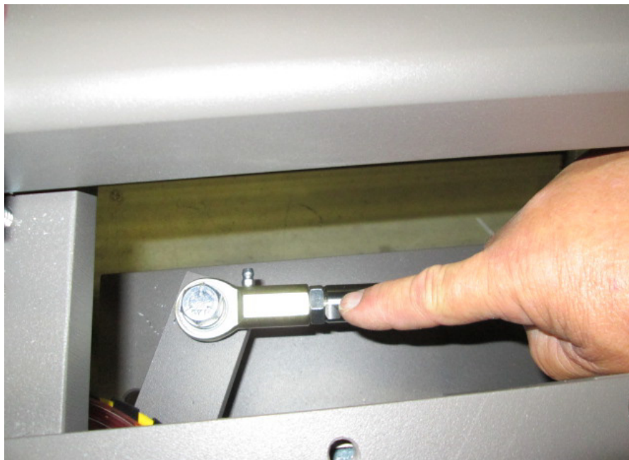
Figure 5 - 3 Check Cylinder Con- Rod For Tightness
