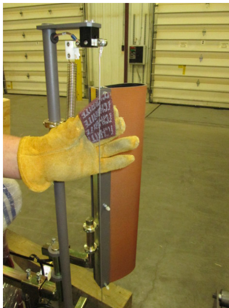
Figure 5 - 1 Cleaning Hot Wire
