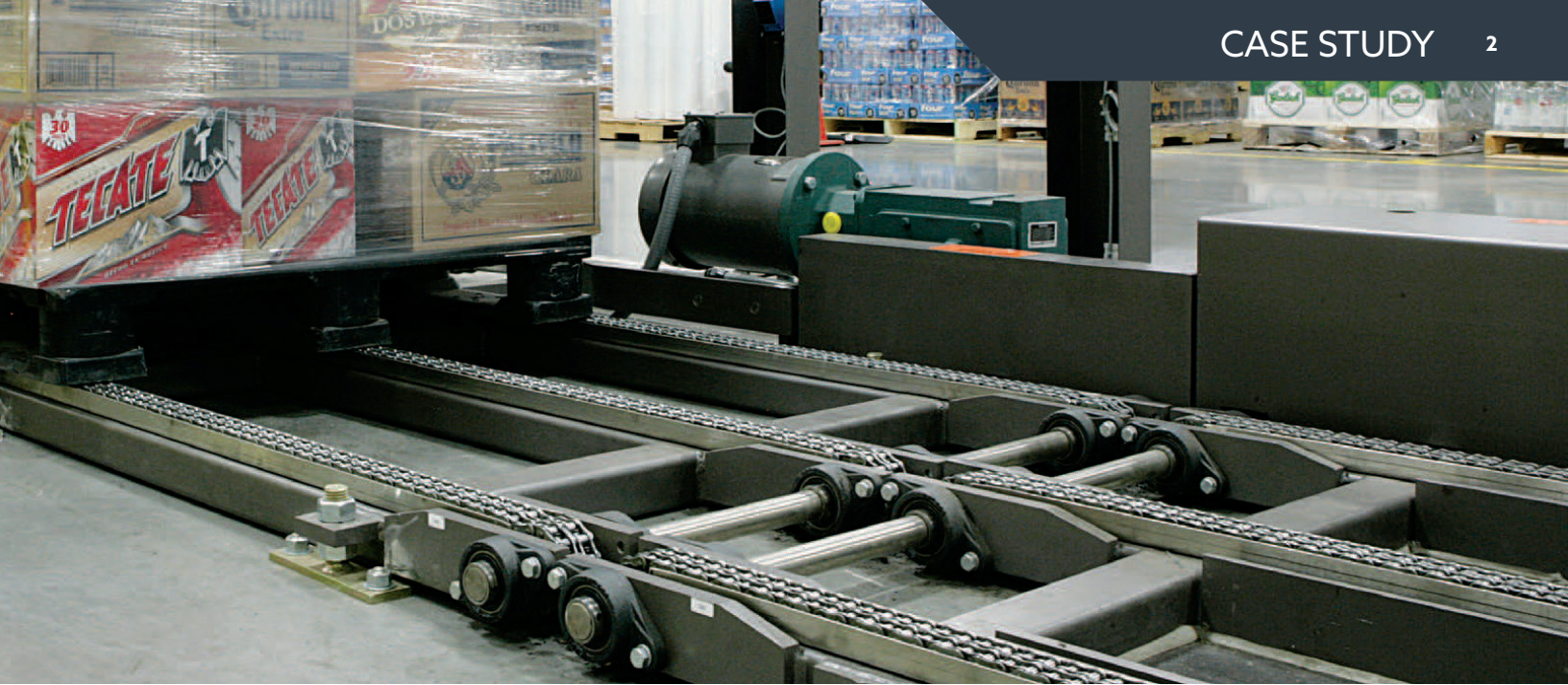
THE SMOOTH CONVEYANCE OF ORION'S HEAVY DUTY DRAG CHAIN CONVEYOR SIGNIFICANTLY REDUCED DOWNTIME DUE TO SPILLED LOADS.
