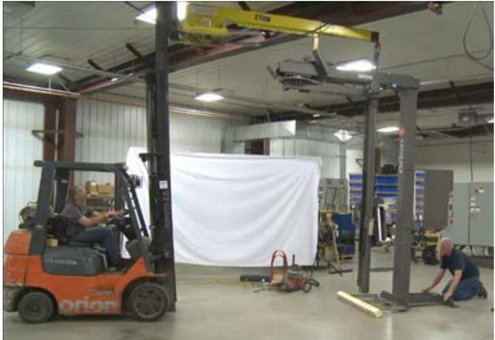
4. Remove the shipping feet while the machine is still held by the lift.
