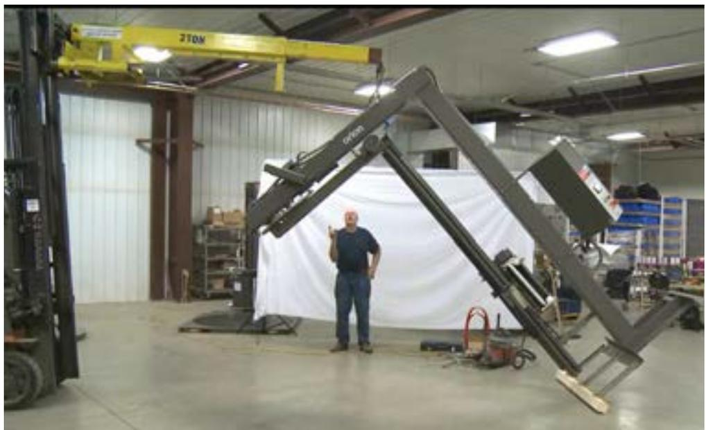
3. Your spotter can position the machine precisely while the lift is holding the tower vertically.
