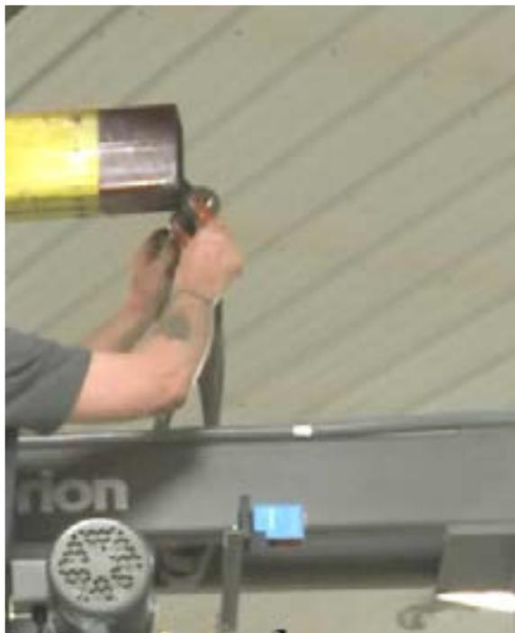
9. Bolt the safety hoop to the bottom of the rotary arm.
