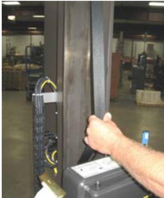
3. Align the limit switch on the inside of the tower with the center of the strap.
