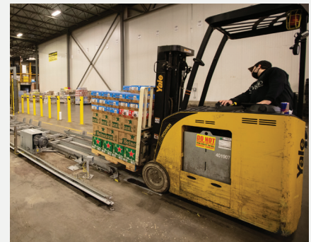
FOUR INCH PASS HEIGHT ALLOWS FOR UNIVERSAL LOADING WITH FORKLIFT, WALKIE, OR PALLET JACK.
