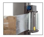
Film carriage pre-stretches film 200% prior to wrapping, reducing the material costs and strengthening the film for a tighter and more secure wrap.
